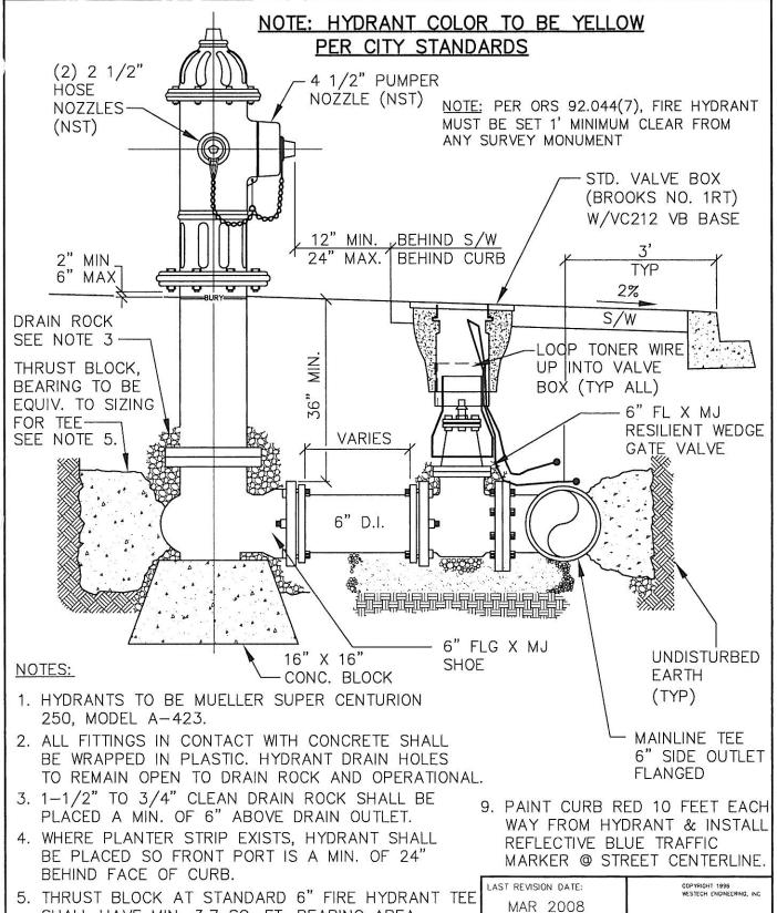
SHALL HAVE MIN. 3.7 SQ. FT. BEARING AREA. 6. ALL HYDRANTS SHALL BE SET PLUMB.
